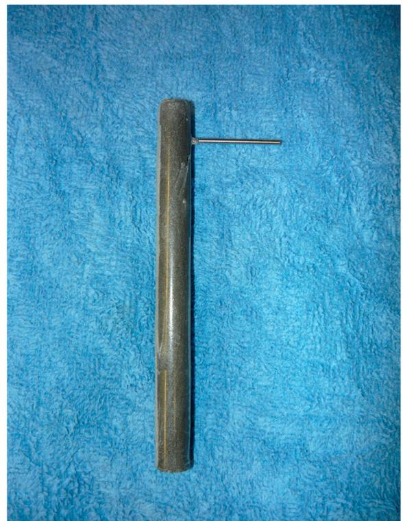
**Figure 1.** Epoxy resin bar (100 mm×9.5 mm) with pin inserted for cyclic load testing. The pin is a 1.6 mm K-wire pin, 50 mm-long, bent at 25 mm and moulded into the middle of the bar with 20 mm of the K-wire exposed for load placement.
