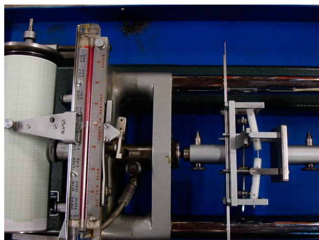
Figure 4. An external skeletal fixator construct in the Hounsfield tensometer 4-point, cranio-caudal bending, test jig. This shows the mercury column and rotating graph paper for plotting the rising mercury column as load is applied. Distracting the load arms applies bending loads to the acetal rod sections as the inner and outer arms move in opposite directions.
